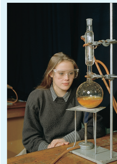
Refluxing is often used for haloalkane substitution reactions with cyanide ions, and haloalkane elimination reactions with hydroxide ions.
