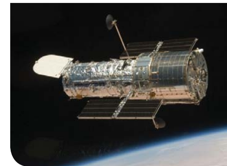
▲ The Hubble Space Telescope uses photocells to transform light energy from the Sun into electrical energy
